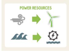
Things that themselves can move/push the generator around, like the wind and moving water for example in a river or a waterfall or in the sea. Here you can see that these resources are harnessed using turbines, as the wind or water flows through the turbine, the blades are specially shaped to capture this flow motion and turn it into a rotational movement.
