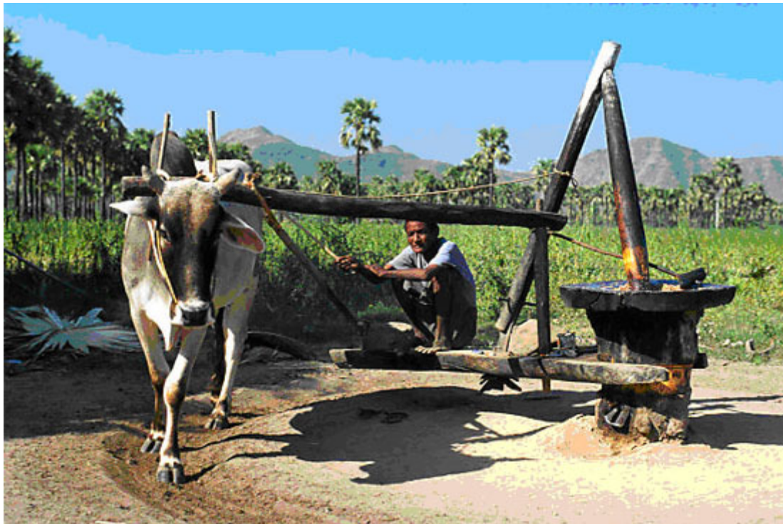
Photograph showing the traditional Oil Milling Process.
